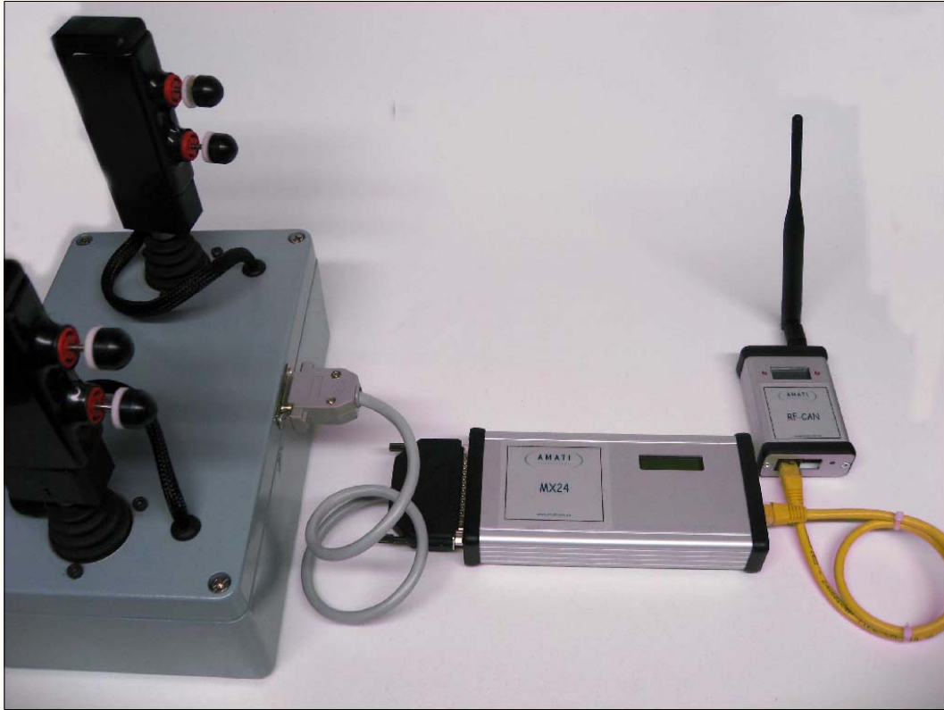
Hand Controls, MX24, RF-CAN Transmitter End
